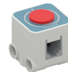
Touch Sensor With two states of press and release
